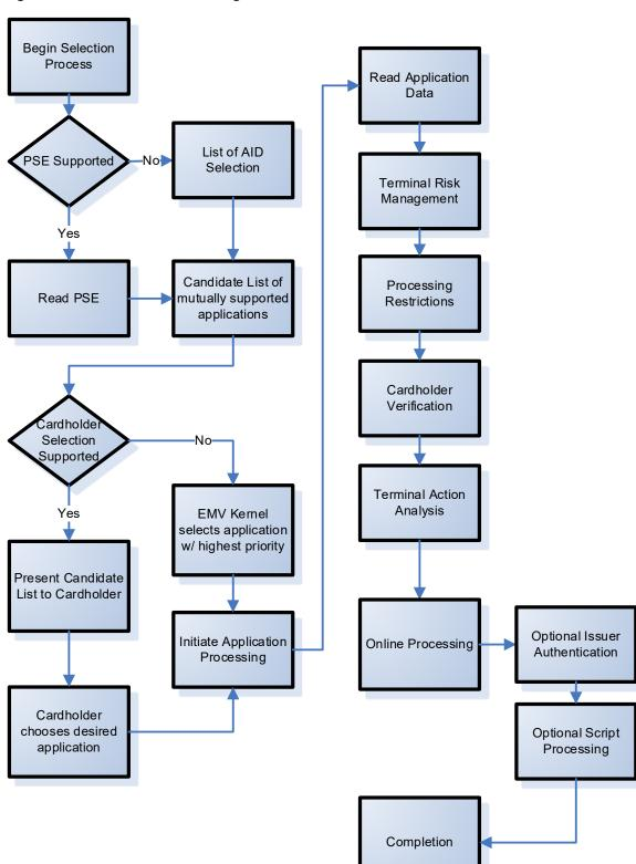
Figure B–1: Basic EMV Terminal Logic
