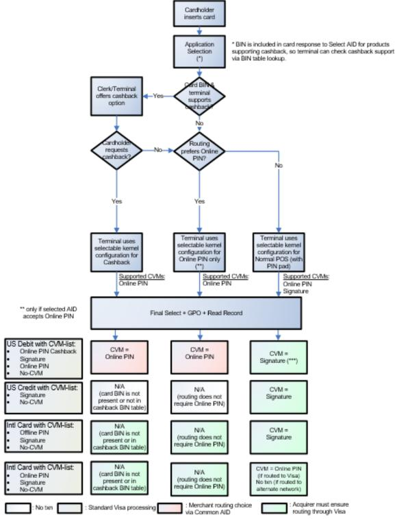
Figure C-4: Combined CVM Processing and Selectable Kernel
